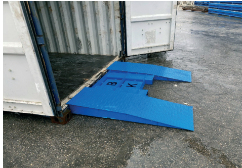
Figure 1. Platform developed to help on unloading moment
