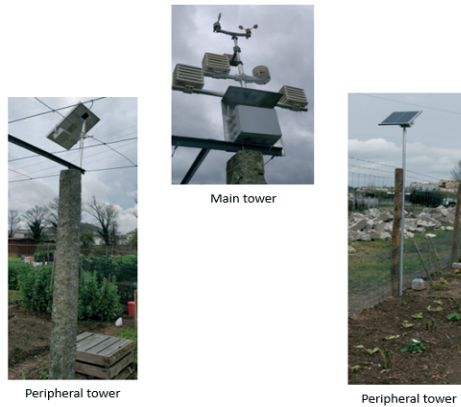
Figure 1: Peripheral towers and main tower responsible for acquiring soil-related and air-related variables, respectively.
