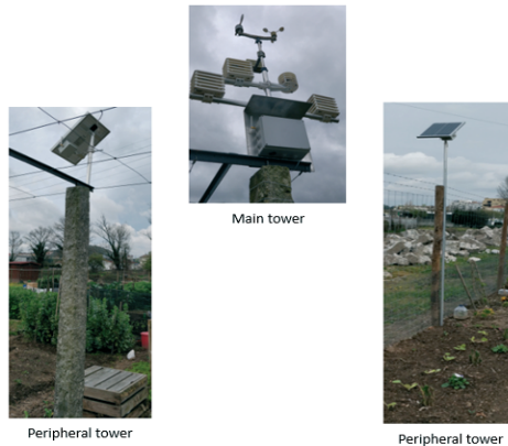
Figure 1: Peripheral towers and main tower responsible for acquiring soil-related and air-related variables, respectively.
