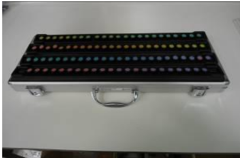
Figura 23: Teste Farnsworth-Munsell 100 Hue Test da Apoloblue
